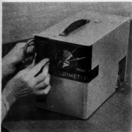
METERED MEASUREMENT is the heart of the Nielsen technique. Audimeters provide a minute-by-minute film record of all set tuning in sample homes, allowing detailed analysis of viewing patterns.
